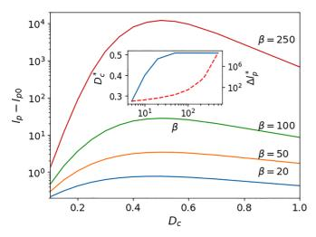
FIG. 2. Persistence length  $l_p$  as a function  $D_c$  and various values of  $\beta$ , where we have subtracted the value  $l_{p0} = 1/3$  reached for  $\beta = 0$ . The inset shows the value of  $D_c$  that maximizes the persistence length as a function of  $\beta$  (solid line), together with the corresponding value of the persistence length  $\Delta l_p^* = l_p^* - l_{p0}$  (dashed line).
